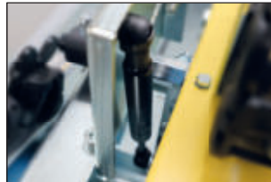
Integrated gas pressure shock absorber guarantees a precise cut.
