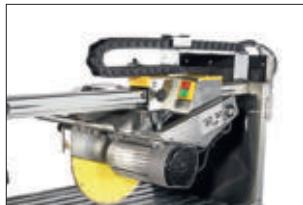
Elegant and practical cable carrier and hose routing.
