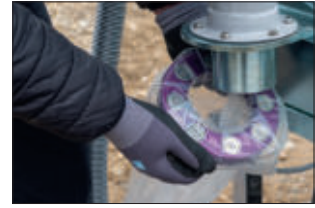
Magnetic holder facilitates the dust bag to be changed within seconds.
