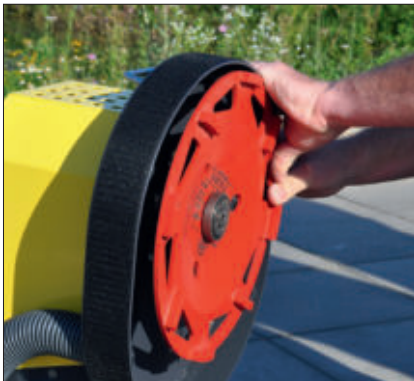
Flexibly mounted drive shaft.
