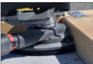
Extraction hood can open, for flush grinding.
