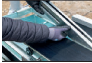
Innovative change channel for simple conversion without using tools.
