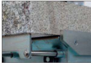
Pull-out table extension for larger materials.
