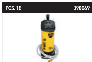
POS. 18 390069 KBZ 700 PWT S Water pressure tank 10 l High-quality construction with stainless steel tank + pressure valve. For carrying out network-independent wet drilling. Water connection suitable for all SAMEDIA core drilling machines and quick-coupling (Gardena), hose connection 1/2".
