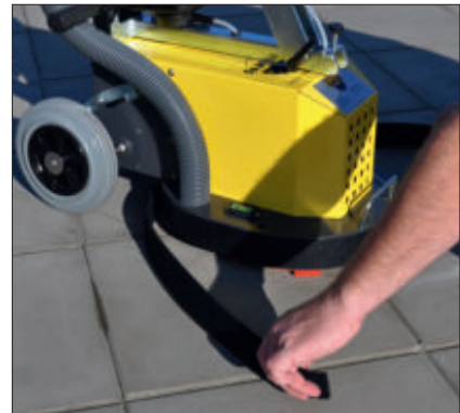
Adjustable, flexible Velcro dust strap.
